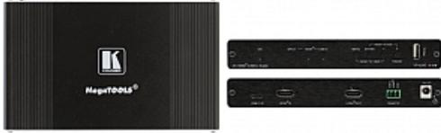
VP-424C is a high-performance digital scaler for HDMI and USB type-C signals. The unit up- or down-scales the selected video signal to resolutions up to 4K@60Hz (4:4:4) at a maximum data rate of 18Gbps (6Gbps per graphic channel). The user selects the HDMI or USB type-C input and the scaled output is sent to the HDMI output
